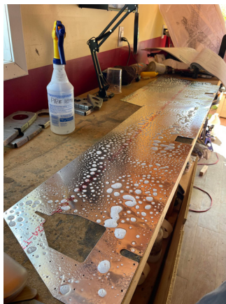
Prepping one of the elevator skins for primer.
